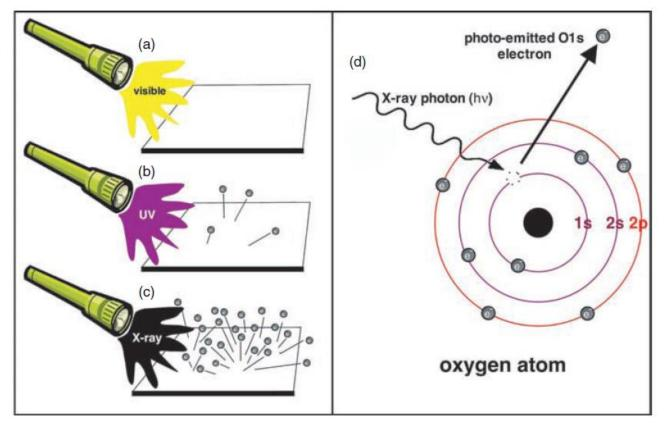
The X-ray photon transfers its energy to a core-level electron imparting enough energy for the electron to leave the atom
