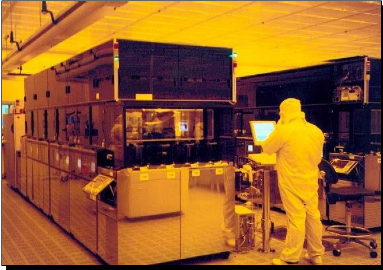
Photo courtesy of Advanced Micro Devices, TEL Track Mark VIII
